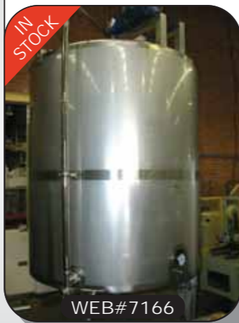
New IOPAK 3000L Mixing Tank (jacketed) with agitator
