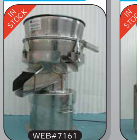
Double Deck 428mm Screen ID s/s Vibratory Screen
